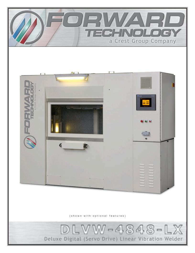
The DLVW-4848-LX is a hydraulic motion controlled digital (servo-electric) drive linearvibration welder capable of welding parts up to 48" x 48" (1219mm x 1219mm) or multiple smaller parts.
