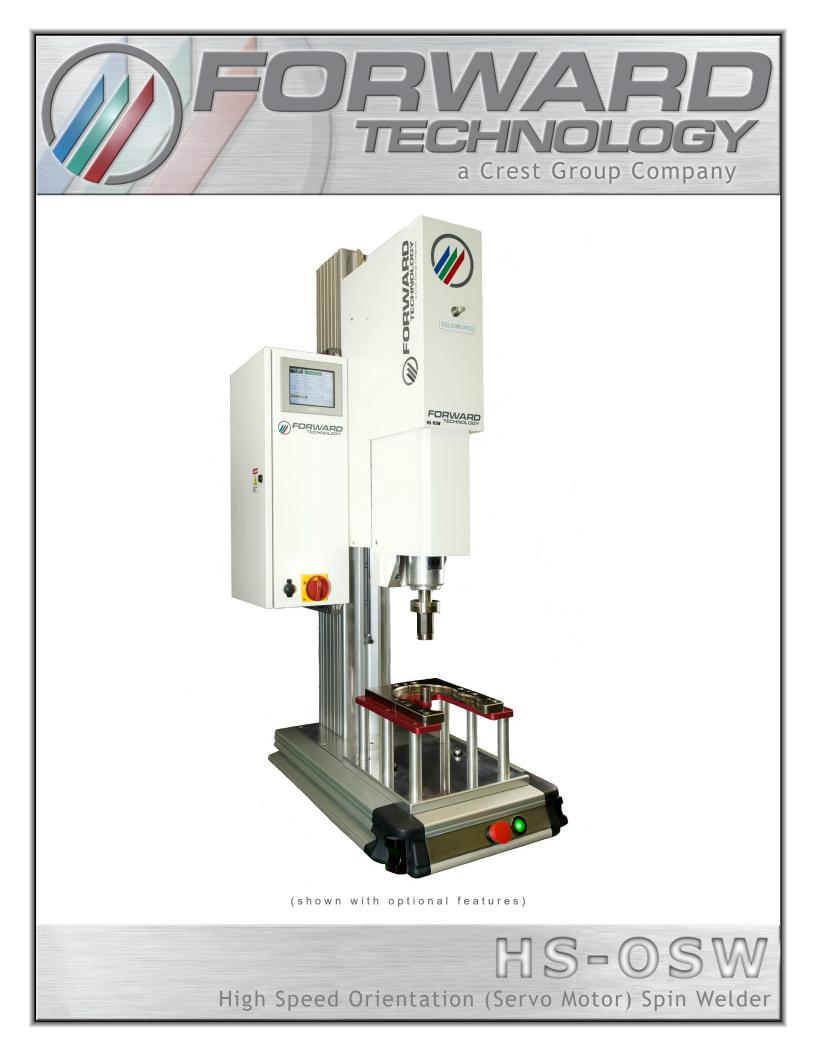
The HS-OSW is a high speed pneumatic motion controlled orientation (servo motor) spin welder designed for smaller diameter, more difficult spin welding applications requiring delivery of high rotational speed while maintaining the highest degree of precision. This servo drive spin welder is capable of orienting part halves relative to each other with a positioning accuracy of +/- 0.5°. Exact start (home) and stop (final orientation) points can be programmed and precisely controlled.
