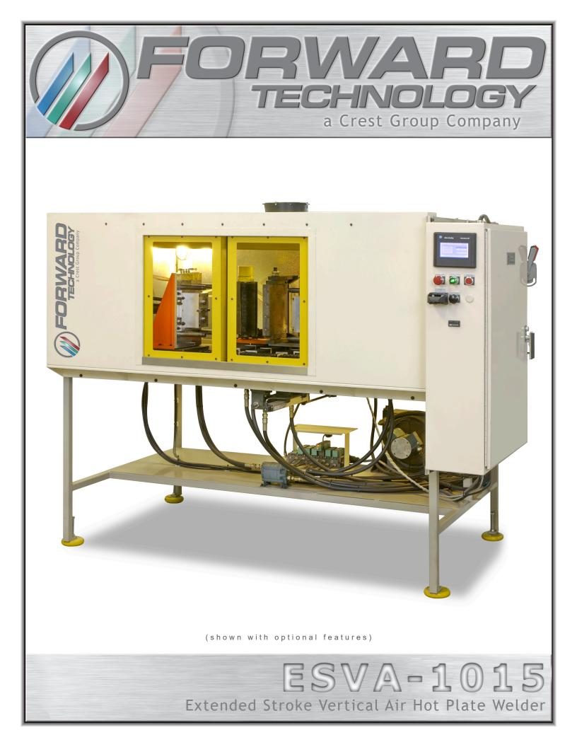
The ESVA-1015 is an extended stroke, vertical heat platen orientation, pneumatic motion controlled hot plate welding system capable of welding parts up to 10" x 15" (254mm x 381mm) or multiple smaller parts. Customized variants of this model are available.
