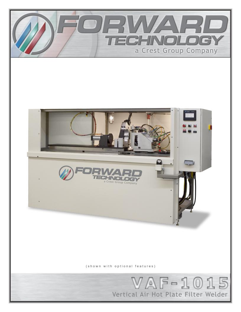
The VAF-1015 is a vertical heat platen orientation, pneumatic motion controlled hot plate welding system specifically designed for welding filter assemblies up to 10" D x 15" H x 69" L (254mm x 381mm x 1753mm). Customized variants of this model are available.
