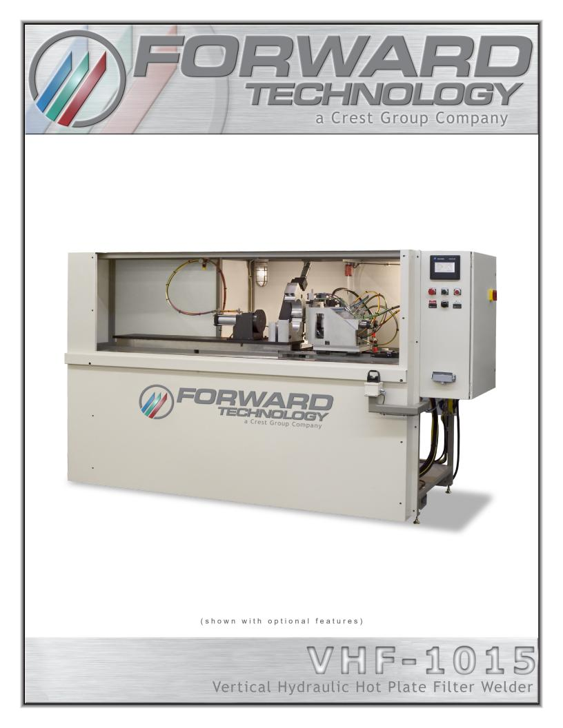
The VHF-1015 is a vertical heat platen orientation, hydraulic motion controlled hot plate welding system specifically designed for welding filter assemblies up to 10" D x 15" H x 69" L (254mm x 381mm x 1753mm). Customized variants of this model are available.
